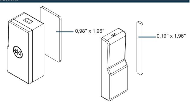
1- Adjust the wall bracket to the surface of your choice, then slide the sensor down on to the mounting fastener on the wall plate until the Snap Lock is secured.
